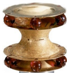
Figure 1.4. Paul's quadrupole and quadrupole ion trap resulted in two of the most used mass analyzers.
