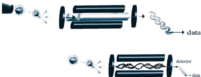
**Figure 2.6.** A linear ion trap mass analyzer confines the ions along the axis of quadrupoles using a 2D radio frequency and stopping potentials on the end electrodes.
