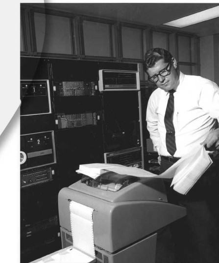
Charles Sweeley examining print out from Digital Equipment Corporation's (DEC) PDP 8/I. DEC computers were used extensively in mass spectrometer data systems.
