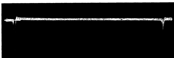
FIG. 2. The eighth order of Rb 85 and Rb 87 on a delayed sweep of 25 \mu\text{sec} at about 950 \mu\text{sec} from the start. The separation is 22 \mu\text{sec} .
