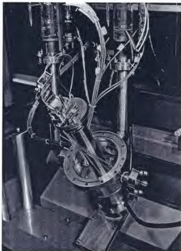
Figure 10. Monoenergetic electron impact ion source used in the Melbourne machine, 1958.
