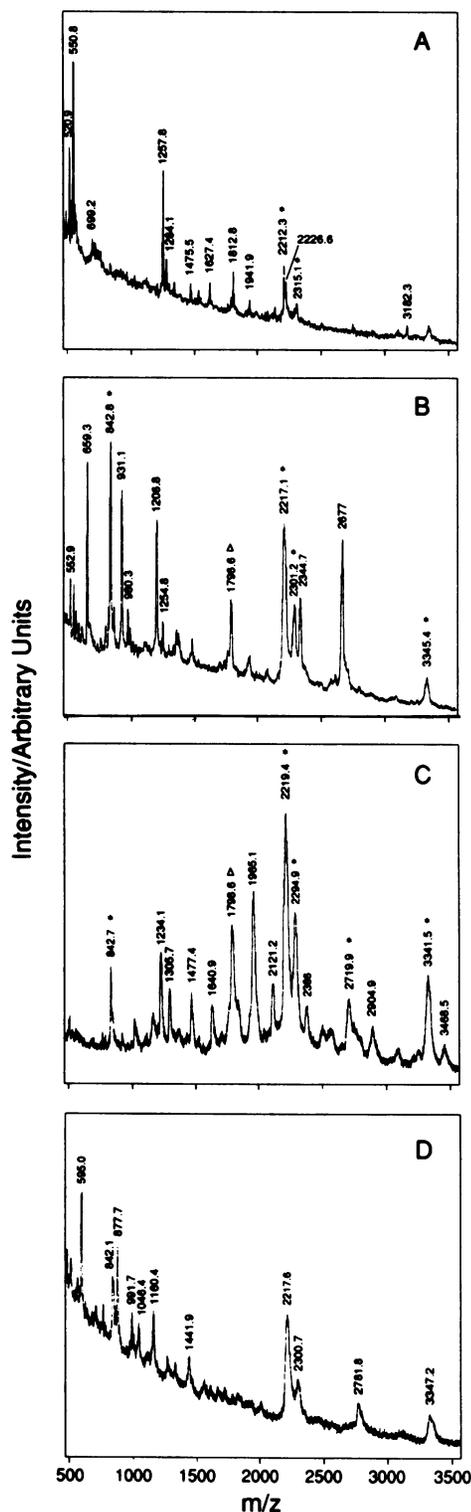
FIG. 2. MALDI mass spectra of *in situ* tryptic digestion of spot 1, cysteine synthase A (A); spot 8, human growth hormone (B); spot 9, 60-kDa elongation factor (C); and a trypsin control (D). Asterisks indicate trypsin autolysis fragments. Peaks marked with  $\Delta$  are unknown contaminants.
