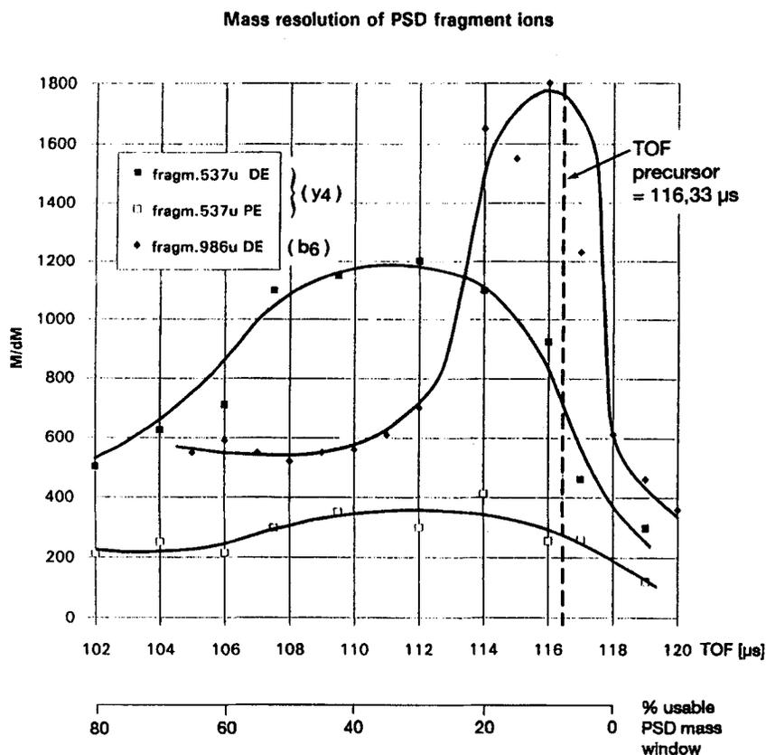
**Figure 5.** Mass resolution of selected PSD fragment ions (precursor: H-VYFYEHFPH-OH) as a function of the flight time (function of the reflectron voltages) in the ReTOF(MS1) instrument. Note the sharp increase of mass resolution around the nominal flight time of the precursor ion.
