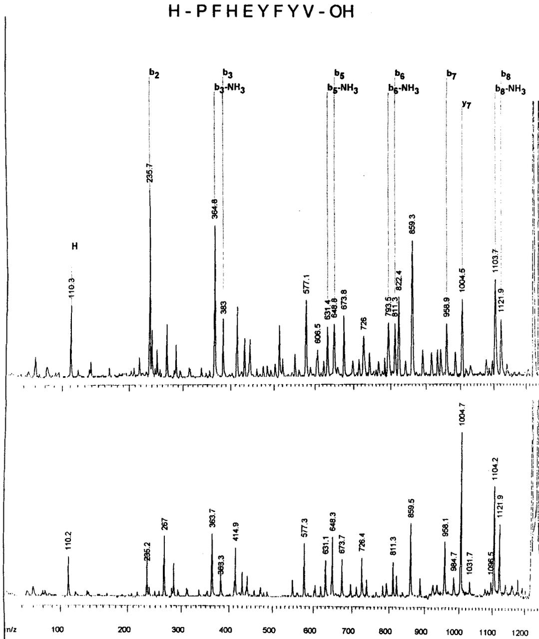
**Figure 7.** Full range PSD mass spectra (compilation of 14 segments with the sum of 50 laser shots each) recorded from a synthetic peptide under PE (top) and DE (bottom) conditions. Only moderate reduction of PSD fragment ion intensities under DE is seen (cf. Fig. 6).
