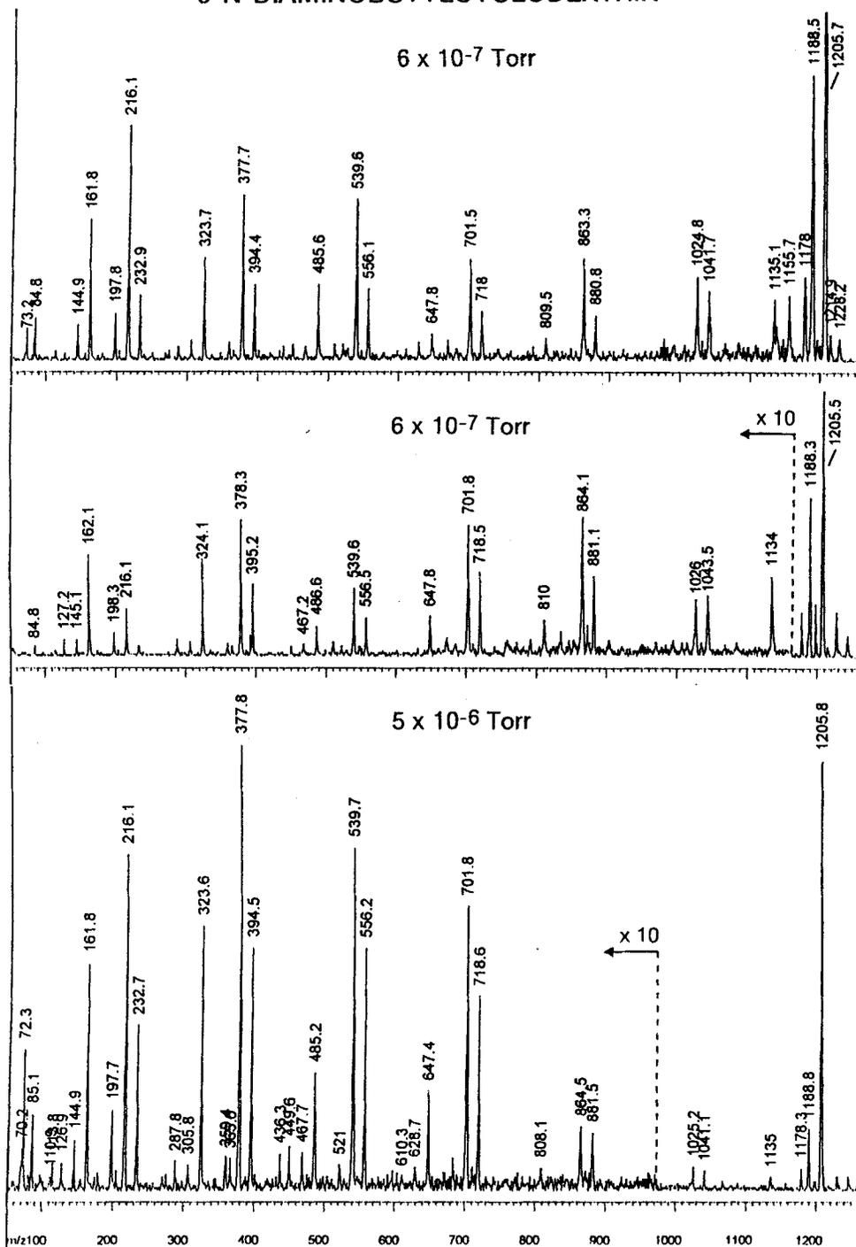
**Figure 9.** Full range PSD mass spectra (compilation of 14 mass segments with the sum of 30 laser shots each) of a cyclic oligosaccharide (3 pmol sample loaded in DHB) obtained under PE (top), DE (middle) and DE in combination with reduced residual pressure (bottom).
