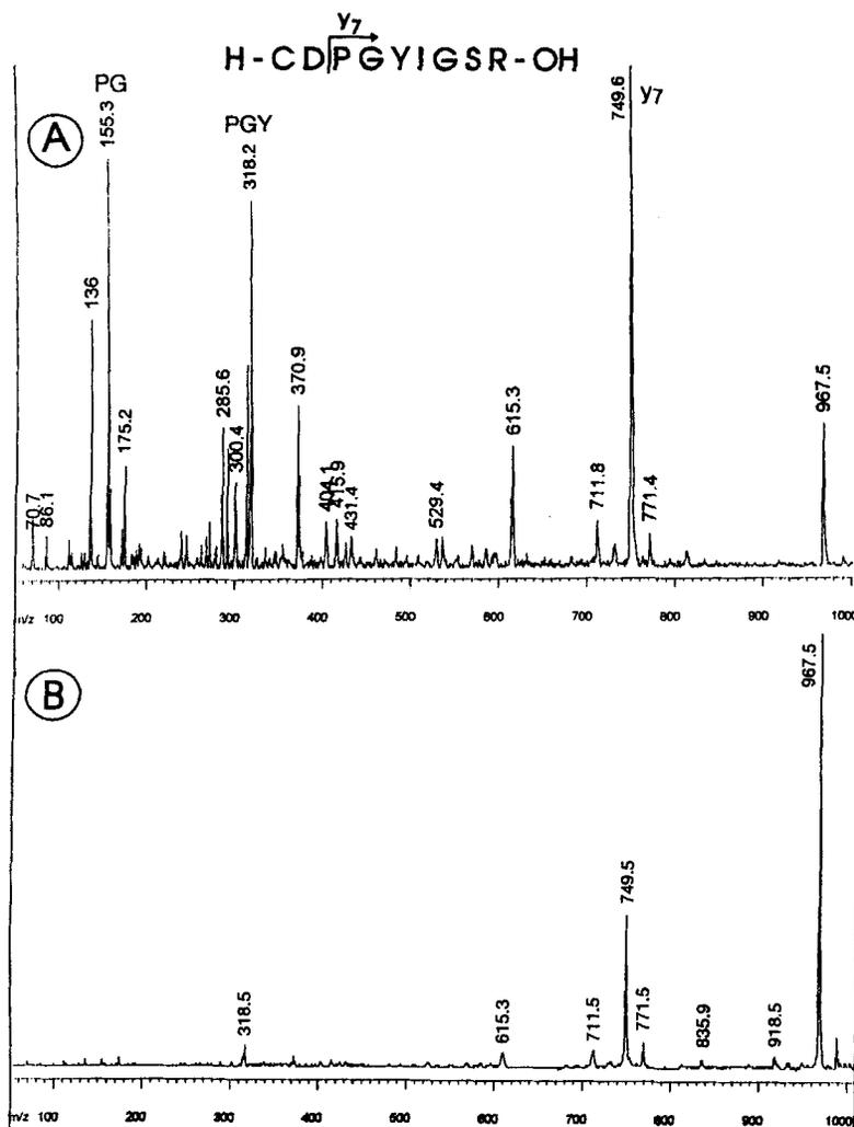
**Figure 6.** Full range PSD mass spectra (compilation of 14 segments with the sum of 50 laser shots each) of a synthetic peptide under PE (a) and DE (b) conditions. Note the complete loss of information at the low mass end of the PSD spectrum recorded under DE conditions.
