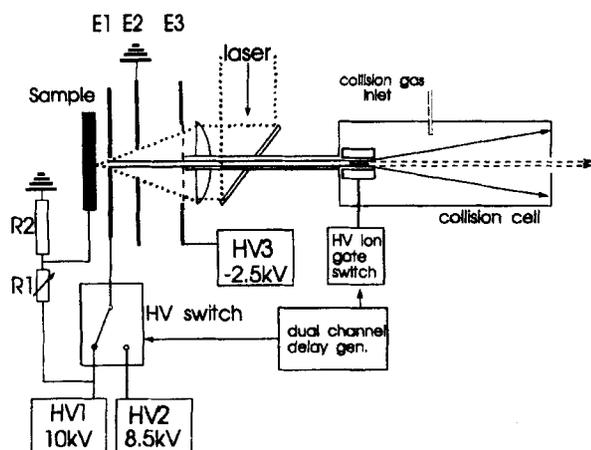
**Figure 1.** Block diagram of the electronics employed for delayed extraction and scheme of the MALDI ion source used in TOF(MS2). See text for further explanation.
