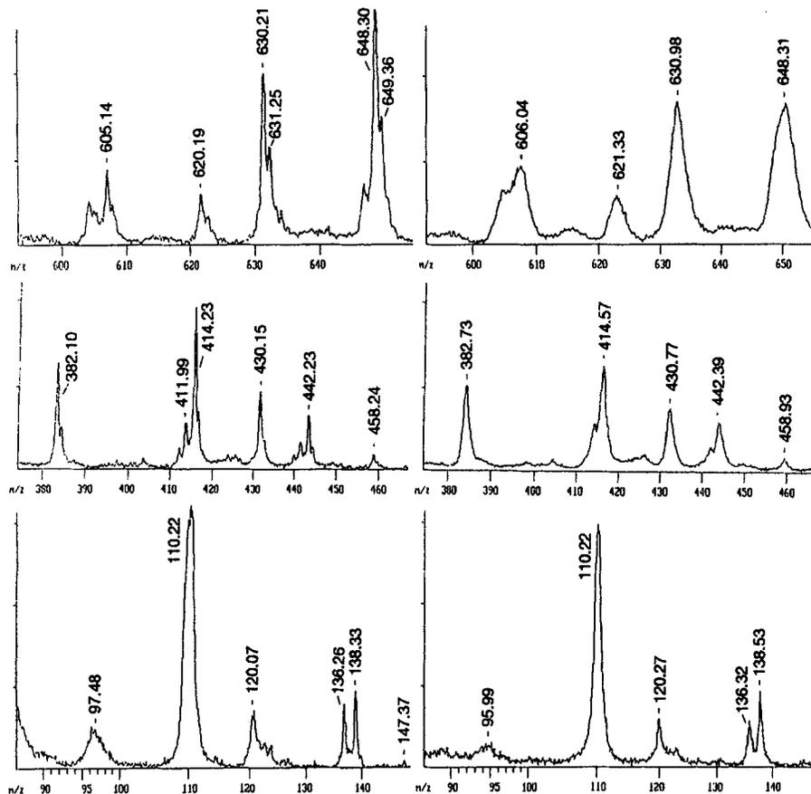
**Figure 8.** Expanded views of various PSD mass windows recorded from the same synthetic peptide as in Fig. 7. The left panel displays spectra (sum of 50 laser shots each) recorded under conditions of DE while the right panel shows the corresponding spectra (on the same y-scale) obtained under PE. See text for further information.
