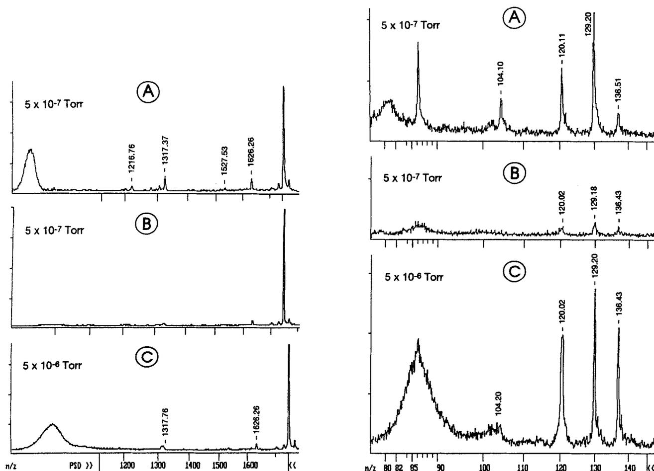
**Figure 3.** High mass (left hand row) and low mass (right hand row) PSD mass window of  $\alpha$ -endorphin recorded under PE (a) and DE (b, c) conditions in ReTOF(MS2) instrument. Note that by an increase of the residual pressure from  $5 \times 10^{-7}$  to  $5 \times 10^{-6}$  Torr the loss of PSD ion yield induced by DE can be counteracted, especially in the low mass range. See text for further explanation.
