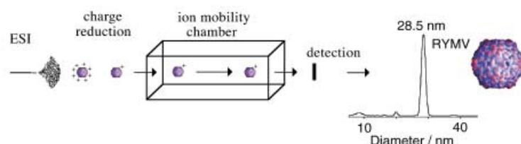
**Figure 4.** Electrospray ion mobility spectrometry provides viral-structure measurements. Charge-reduction electrospray ionization coupled with ion mobility spectroscopy measures the gas-phase quaternary structure of particles. The ESI ion mobility spectrum of RYMV demonstrates a monodisperse peak of ions of the expected diameter (based on the virus's crystal structure).
