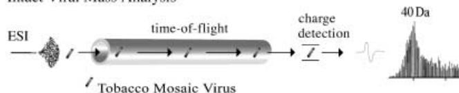
**Figure 3.** Intact-virus analysis achieved with a TOF charge-detection mass spectrometer. The successful mass measurement of an intact virus particle ultimately required the use of an instrument combining electrospray ionization, TOF mass analysis, and a novel charge-detection device designed by Benner.
