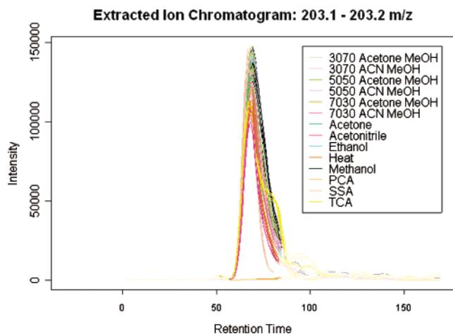
**Figure 1.** EIC generated by XCMS for enhanced metabolite feature visualization. The title of each EIC shows the  $m/z$  range of the feature being plotted, where the  $x$  and  $y$  axes show retention time (in seconds) and intensity, respectively. The color of each EIC can be chosen so that different sample groups can be distinguished.
