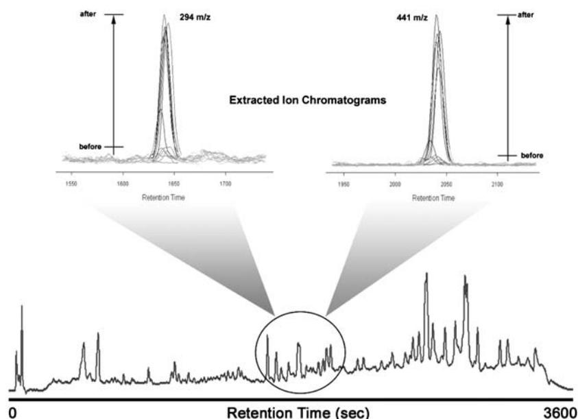
Figure 3. Distribution of newly detected metabolite features after MTBE treatment and PLC using the cerium-modified column.
