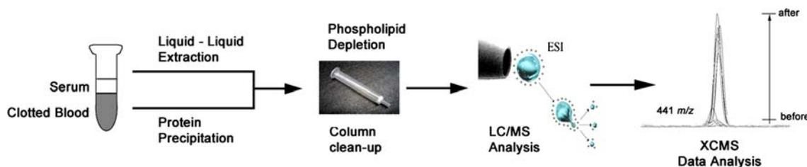
Figure 2. Overview of the sample processing steps employed for PLC using cerium-modified columns. Serum samples were prepared as shown in tables 1, 2 and analyzed using LC/MS. Serum metabolite profiles were compared using XCMS data analysis in order to evaluate the effects of different solvent systems on phospholipid capture.
