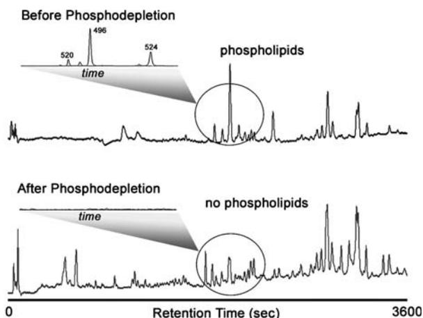
Figure 6. Chromatograms of MTBE extracted serum with (A) no PLC and (B) PLC using a cerium-modified column. Inset, the EICs of the major phospholipids at  $m/z$  496, 520 and 524 show that they have been depleted after treatment. New metabolite features can be seen throughout the chromatogram.
