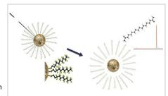
Schematic illustration of the possible desorption mechanism. On irradiation, the gold core efficiently absorbs the laser energy
