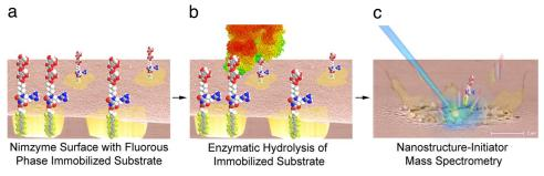
Fig. 1. Illustration of the Nimzyme assay. (a) Immobilization of metabolites in the fluorous "clathrate" phase of the NIMS surface. (b) Incubation of the surface with the sample to screen for enzymatic activity. (c) Laser irradiation, resulting in vaporization of the fluorous phase, efficiently transferring the immobilized substrate and products into the gas phase.
