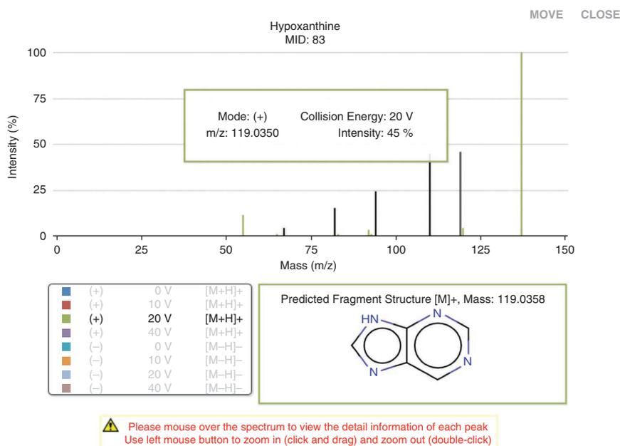
Stage 2: If a co-eluting metabolic peak is within 1–2  $m/z$  of your ion of interest, it may provide a convoluted spectrum. If you suspect that this is the case, you should refragment this species with a narrower isolation window. If it is within 1 Da, this may not be sufficient to isolate the species, and you may need to use another approach to identify this peak. If two ions are co-eluting, different chromatographic conditions may allow these two species to be separated as in **Figure 2**.
