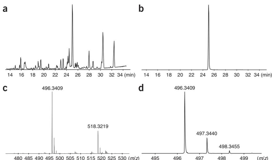
**8** | By using the Range Select cursor, zoom in on the MS spectra as in **Figure 1c**. Determine the adduct of your peak. In this case, 496.3409 is likely  $[M + H]^+$ , as a peak of  $\sim 22$  Da (518.3219) is present, which would correspond to the  $[M + Na]^+$ .
