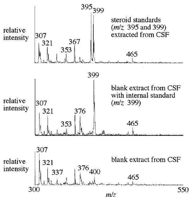
Figure 1. NanoESI mass spectra using precursor ion scanning of sulfate compounds recovered from human CSF by the two-step extraction method. (top) Extract from CSF blank spiked with pregnenolone sulfate ( $m/z$  395) at 250 fmol/ $\mu$ L, and the internal standard pregnenolone- $d_4$  sulfate ( $m/z$  399) at 250 fmol/ $\mu$ L. (middle) Extract from CSF blank with internal standard pregnenolone- $d_4$  sulfate ( $m/z$  399) at 250 fmol/ $\mu$ L. (bottom) Extract from CSF blank.
