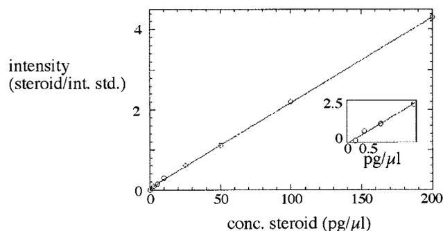
Figure 2. Standard curve of pregnenolone sulfate with internal standard, pregnenolone- $d_4$  sulfate, generated using precursor scanning with negative ion nanoESI. Quantitative data obtained in separate calibration experiments ranging from 100 amol/ $\mu$ L to 500 fmol/ $\mu$ L (40 fg/ $\mu$ L–200 pg/ $\mu$ L). The limit of quantitation was 250 amol/ $\mu$ L where the accuracy was found to be within  $\pm 20\%$ .
