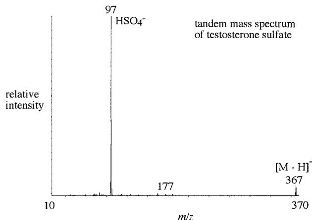
Figure 4. Negative ion nanoESI MS/MS spectrum of testosterone sulfate ( $m/z$  367) from extract of male bonobo urine. Base peak ( $m/z$  97) is the sulfate anion  $[\text{HSO}_4]^-$ .
