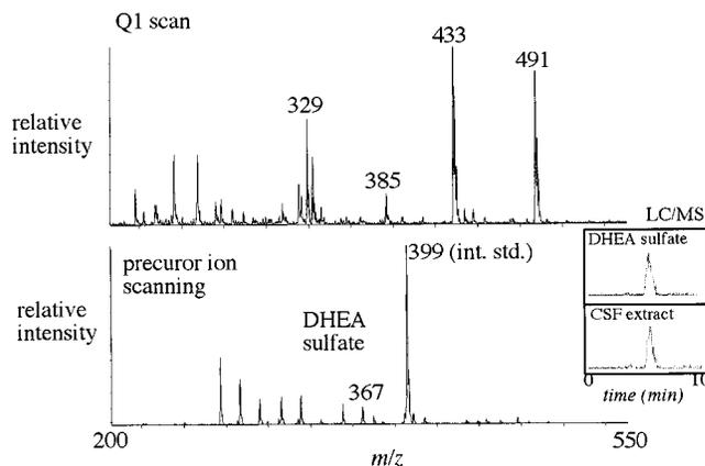
Figure 7. Negative ion nanoESI Q1 scan (top) and precursor ion scanning mass spectral data of steroid sulfates extracted from CSF (pregnant human) containing an internal standard ( $m/z$  399) at 1.2  $\text{pmol}/\mu\text{L}$ . The DHEA sulfate anion was detected at  $[M - H]^- = m/z$  367 and estimated at 100  $\text{fmol}/\mu\text{L}$ . The selected ion chromatogram of DHEA sulfate standard (inset, top) and a sample extracted from an actual CSF sample (inset, bottom) are shown.
