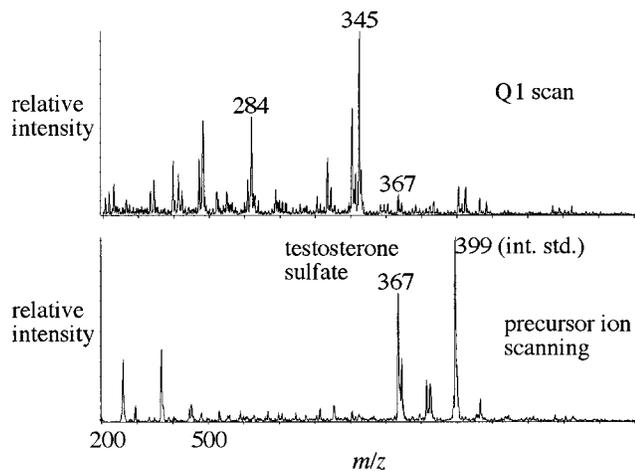
Figure 3. Mass spectra of male bonobo urine extract, obtained by negative ion nanoESI. Q1 scan (top) and precursor ion scan (bottom) was used for steroid sulfates and the internal standard ( $m/z$  399) at 12.5 pmol/ $\mu$ L. Testosterone sulfate detected at  $[M - H]^- = m/z$  367 and estimated at 9.5 pmol/ $\mu$ L.
