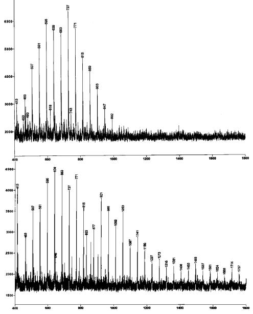
FIG. 9—DIOS mass spectrum from liquid contained in a SLIP<sup>®</sup> PLUS bottle provided by the manufacturer (top), and the liquid from the SLIP<sup>®</sup> PLUS bottle provide by the suspect. At trial his attorneys stipulated their client had added some of the Encare<sup>®</sup> product to the bottle.
