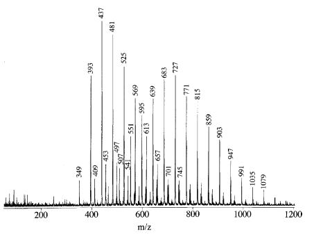
FIG. 5—DIOS mass spectrum of PEG lubricant [peak grouping with 437 Da (n=9) maximum and 44 Da between adjacent peaks) and nonoxynol-9 spermicide [peak grouping with 727 maximum (n=11) and 44 Da between adjacent peaks] from a Ramses<sup>®</sup> Extra spermicidally lubricated condom. \*Used with permission from Fig. 4, Thomas JJ, et al., Analytica Chimica Acta 2001;442:183–90, Elsevier Science.
