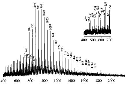
FIG. 6—DIOS mass spectrum from a swab extract from a volunteer immediately following the use of an Encare® vaginal contraceptive insert. Nonoxynol-9 peaks are buried within the low mass side of the PEG spectrum (peaks at 463, 507, 551, 639, and 683 Da in the insert on the upper right). \*Used with permission from Fig. 5, Thomas JJ, et al., Analytica Chimica Acta 2001;442:183–90, Elsevier Science.
