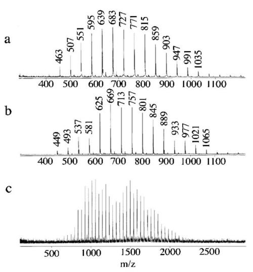
FIG. 4—DIOS–MS spectra of: (a) nonoxynol-9 (nonylphenylpolyethylene glycol); (b) octoxynol-9 (octylphenylpolyethylene glycol); and (c) a mixture of PEG 1000 and PEG 1500. \*Used with permission from Fig. 3, Thomas JJ, et al., Analytica Chimica Acta 2001;442:183–90, Elsevier Science.
