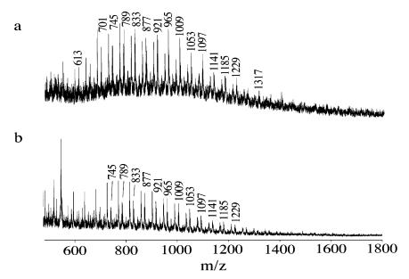
FIG. 7—DIOS mass spectrum showing a pattern of PEG in the same range as the Encare<sup>®</sup> product. Samples taken from: (a) deep vaginal swab from alleged victim, and (b) penile (glans and shaft) swab from suspect. \*Used with permission from Fig. 6, Thomas JJ, et al., Analytica Chimica Acta 2001;442:183–90, Elsevier Science.
